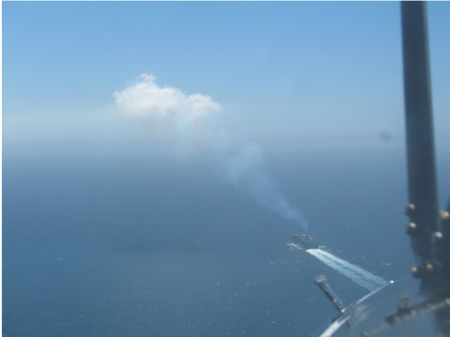
Ship stack smoke initiating cloud formation by injecting fine particles above the marine boundary layer
